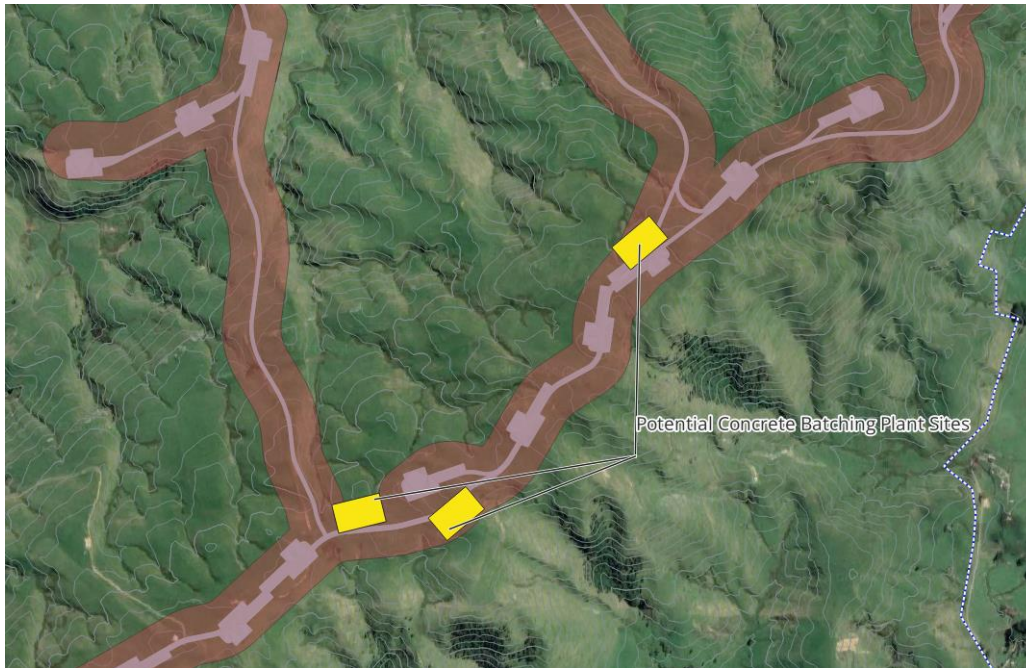
Figure 8.1: Potential Concrete Batching Plant Sites
